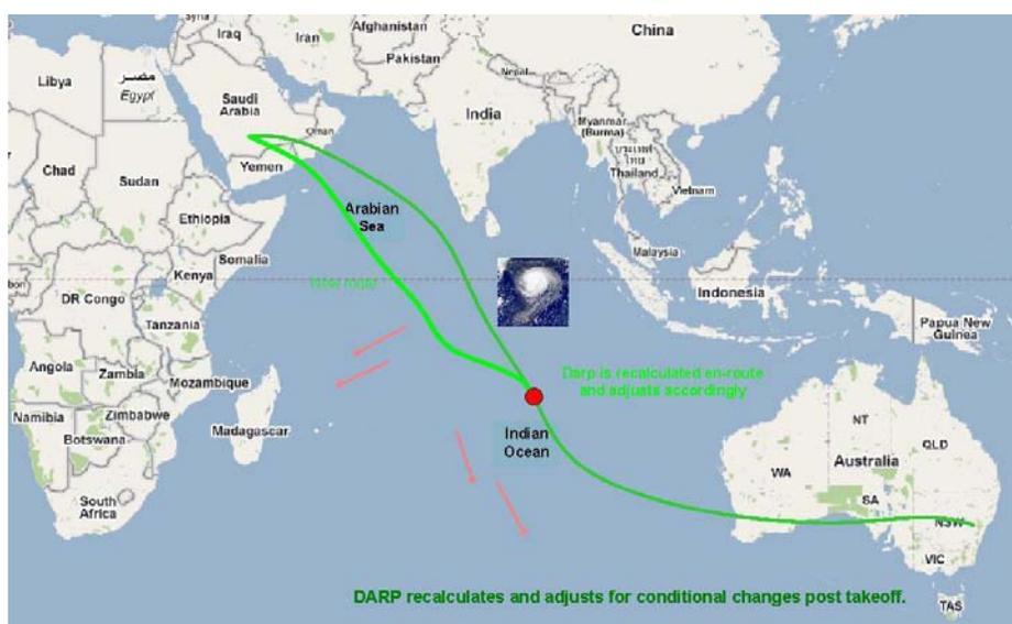
**Figure 2 - Dynamic Airborne Reroute Procedure Example**
