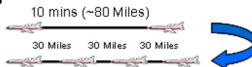
**Figure 3 - Reduced Oceanic Separation Minima**
